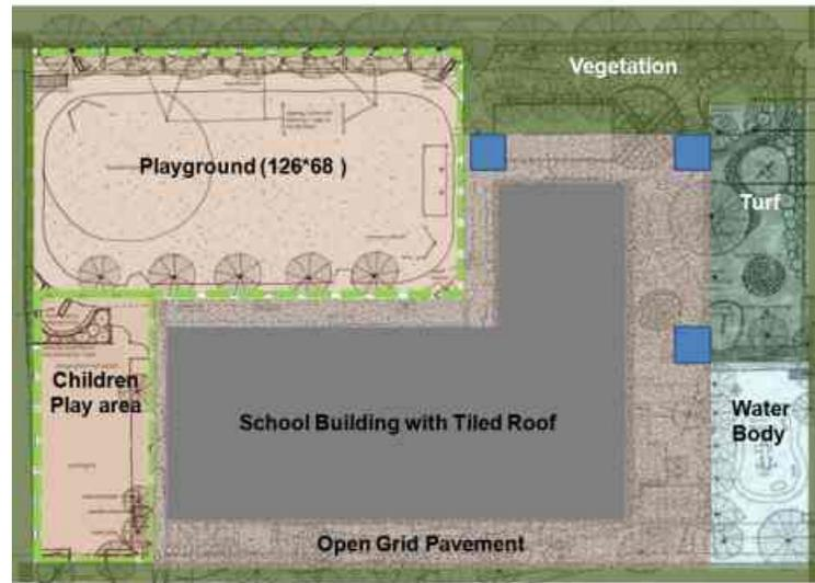
Site plan highlighting the different surface types
